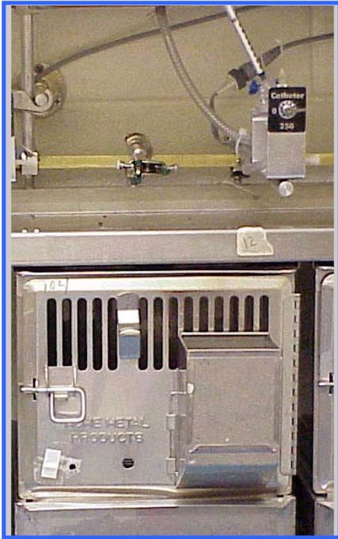
**Figure 3:** Close-up of transducer used for blood pressure measurements. Special valve permits calibration procedure to be performed on all transducers at once.
