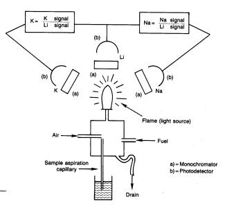
light is detected through wavelength filters (monochromator) and converted to an electronic signal (photodetector) proportional to the concentration of atoms in the sample. Cesium (Cs) is used in the dilution buffer as an internal standard to account for any fluctuations in air or flame. Concentration is calculated by comparing a ratio of standard (calibrator) emmission to the ratio of emission from the internal standard, which should remain constant.
